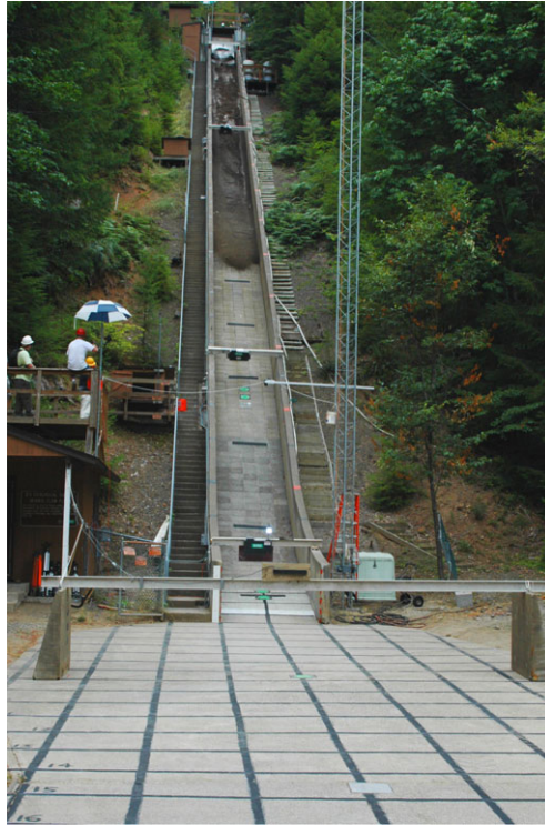
Figure 3. Photograph of the US Geological Survey debris-flow flume in Oregon, USA. The flume is 95 m long and 2 m wide. Most of the bed slopes uniformly at 31^\circ . The photograph shows a 10 \text{ m}^3 gate-release flow, with the flow front at x \approx 53 \text{ m} downslope from the headgate approximately 5.3 s after the gate opened [15].
