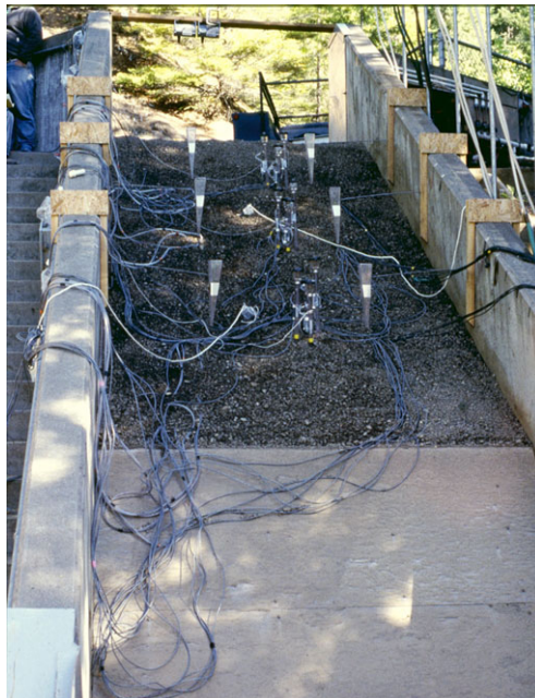
Figure 4. Photograph illustrating the initial condition of a 6 \text{ m}^3 sediment prism in a debris-flow mobilization experiment conducted at the US Geological Survey debris-flow flume on 6 June 1999. Sediment is held in place by a bed-normal retaining wall. See Iverson et al. [14] for details.
